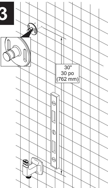
Mark the placement of the upper mounting base plate holes using a level in a vertical line from the lower mounting base. Use upper mounting base plate (1) as a guide. Vertical distance is 30" (762 mm) between centers.
