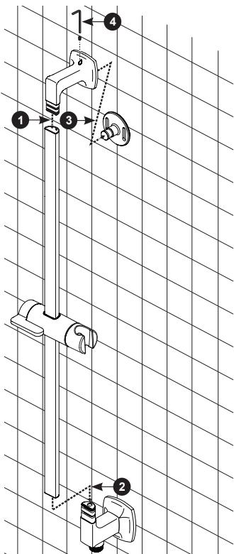
**C.** Note: The holder can be reversed by pressing the lever down and sliding it off the bar. Turn the holder upside down, and slide it back on the bar. With lever still depressed, slide to position and release.
